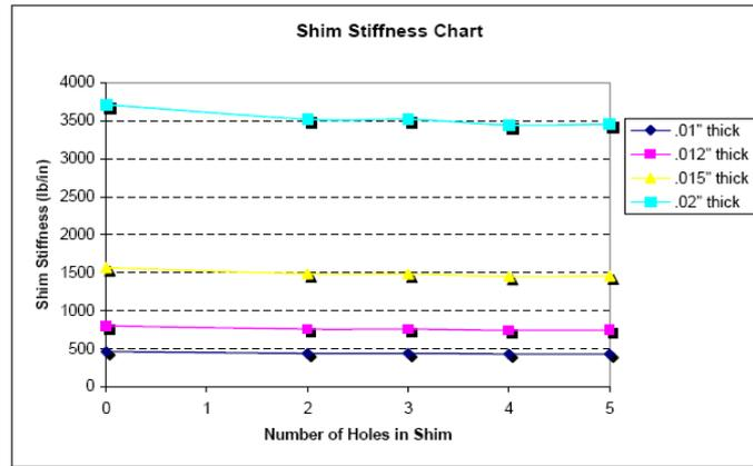
Figure 6: Shim Stiffness Chart for Varied Shim Thickness
