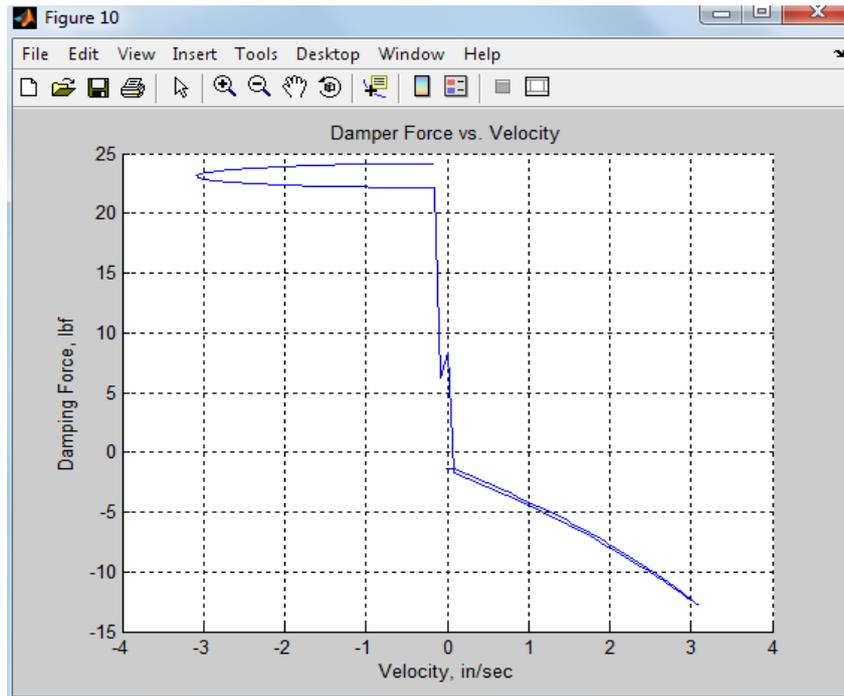
**Figure 9: Plot of Damping Force and Piston Velocity**
