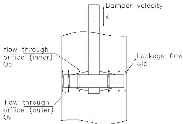
Figure 3: Oil Flow in the Fluid Damper
