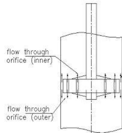
**Figure 2: Oil Flow in the Fluid Damper**
