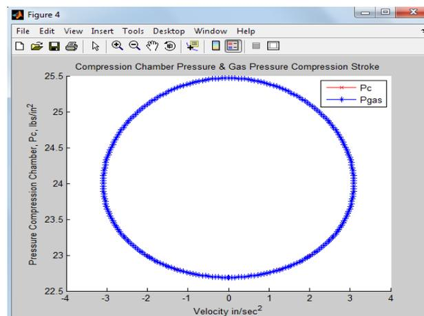
Figure 8: Plot of Compression Pressure and Piston Velocity
