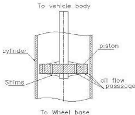
**Figure 1: Construction of Fluid Damper Used Automobile Shock Absorber**
