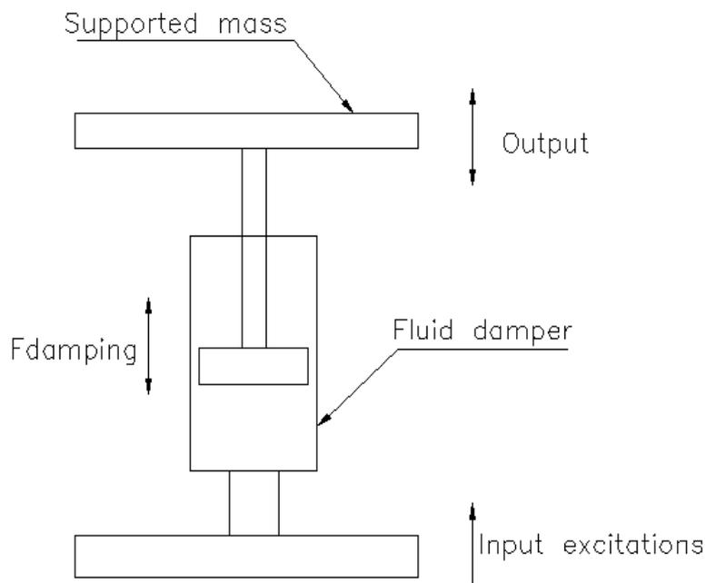
**Figure 10: Single Degree of Freedom Model in Matlab**
