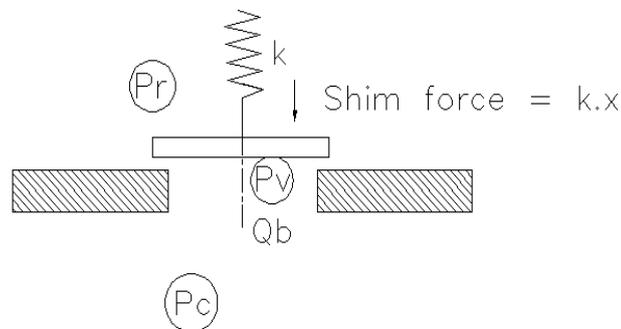
Figure 7: Oil Flow through Inner Orifice
