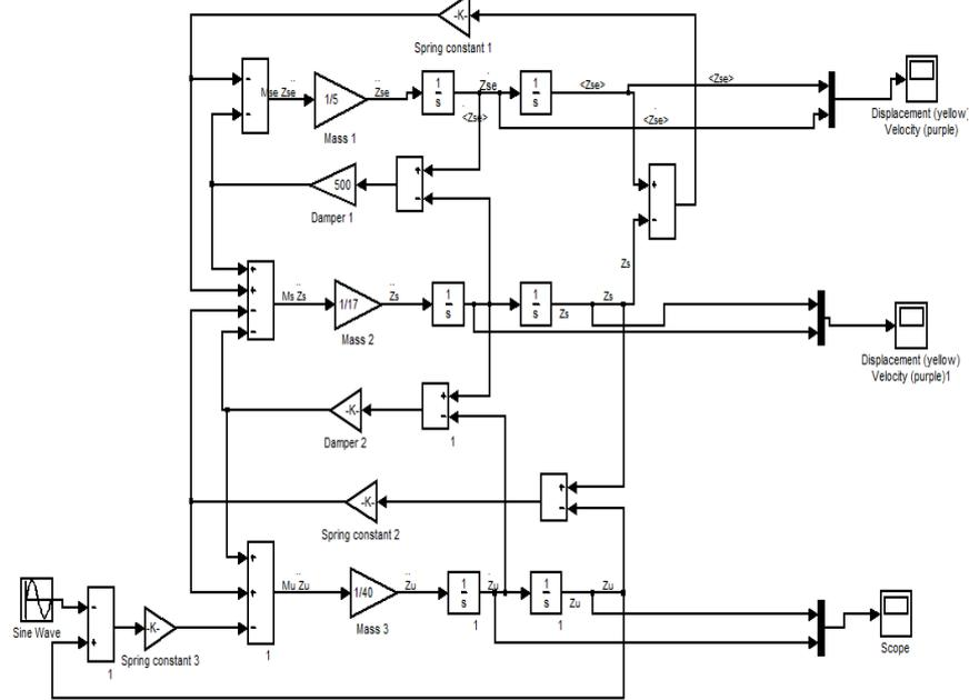
**Figure 11: Matlab Simulink Model of the Fluid Damper**
