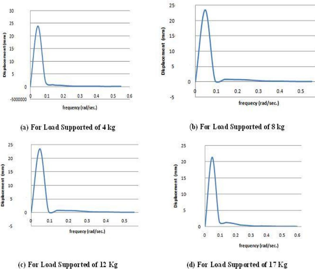
**Figure 12: Simulation Results for Displacement at Supported Mass at 1 Hz Frequency**
