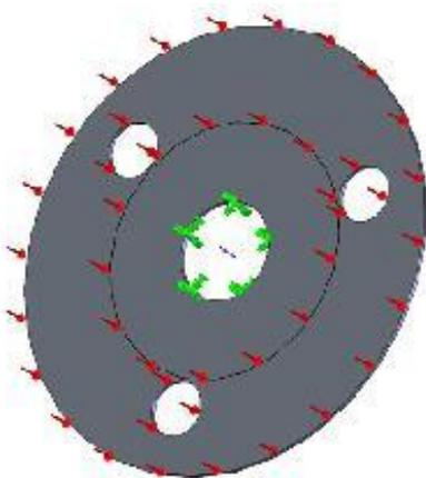
Figure 4: Pressure Applied on the Shim
